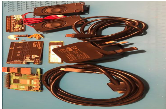
Figure 11. The main parts of the system, including the power supply, speakers and processing unit (namely the Raspberry Pi)
