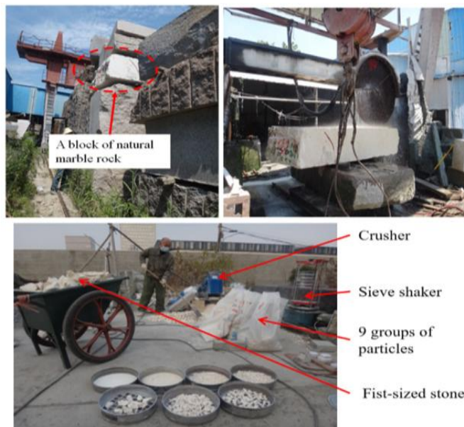
Figure 14. In the experimental setup, a large block of natural marble rock was initially cut into smaller pieces using a special saw, and then further broken down into fist-sized stones manually.
