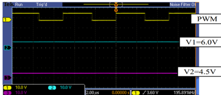
Figure 22. Output voltages of SIDO buck-buck converter [21] ©IEEE.
