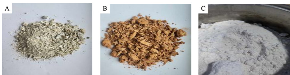
Figure 4. (A). female calcite purification processed by burning at 600 °C (Manba Datsan Pharmaceutical Factory); (B). female calcite purification processed by burning at 600 °C (Manba Datsan Pharmaceutical Factory); (C). male calcite purification processed by burning at 600 °C (Mongem Pharm Pharmaceutical Factory).
