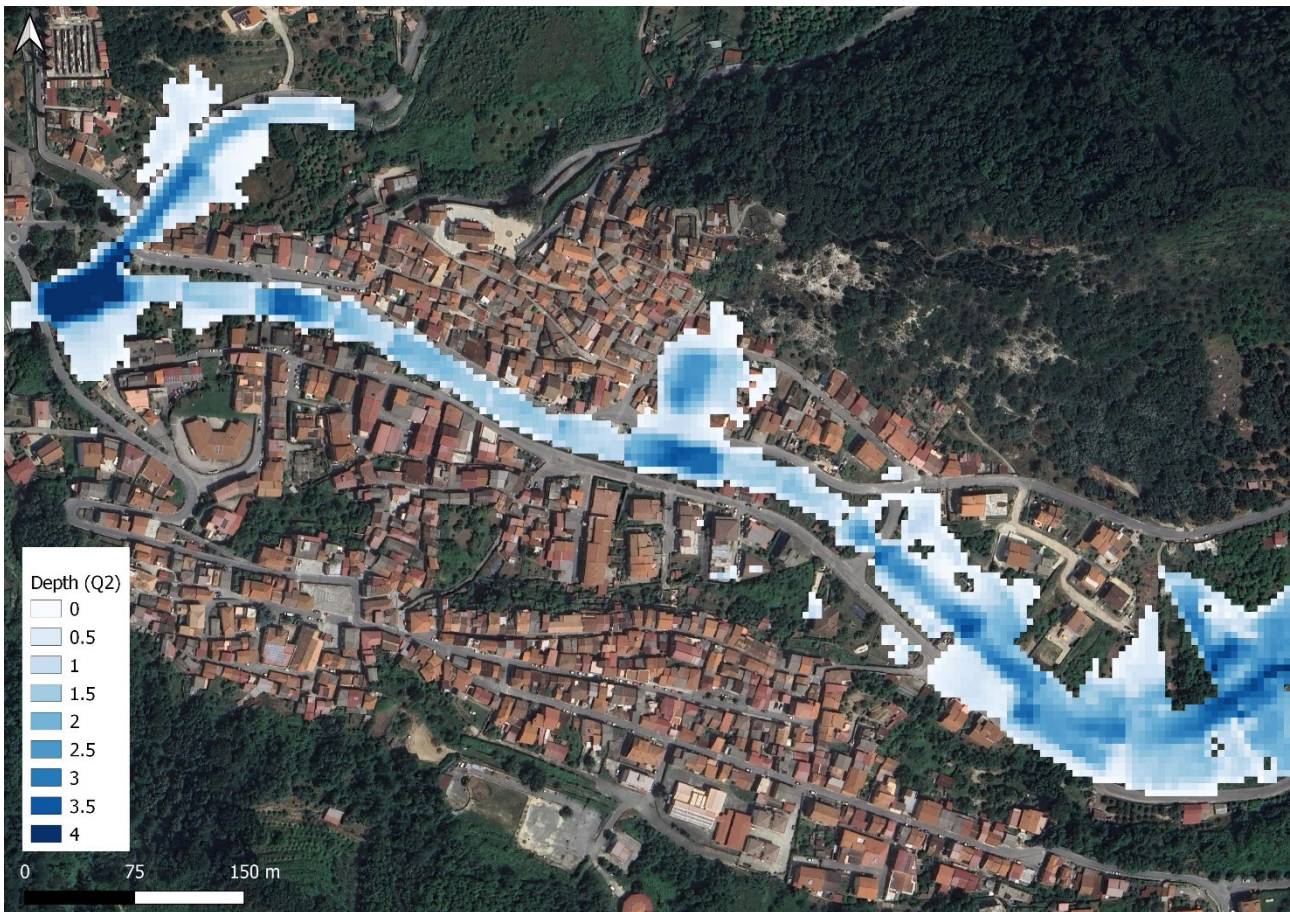
Figure 7. Floodable areas downstream of the Metramo dam related to Q2 scenario added to the QAm max threshold.
