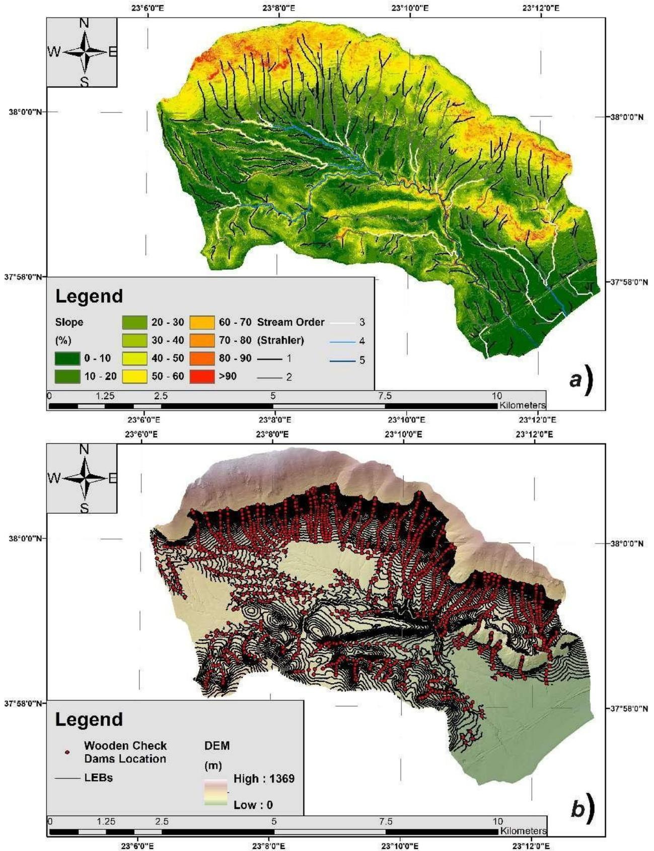
**Figure 6.** Designing the proposed works. (a) The stream order and slope were calculated based on the area's DEM within GIS, and together with the burn severity areas (as shown in Figure 4), to guide us in designing the PFPs; (b) The final map with the locations of the designed LEBs and wooden check-dams.
