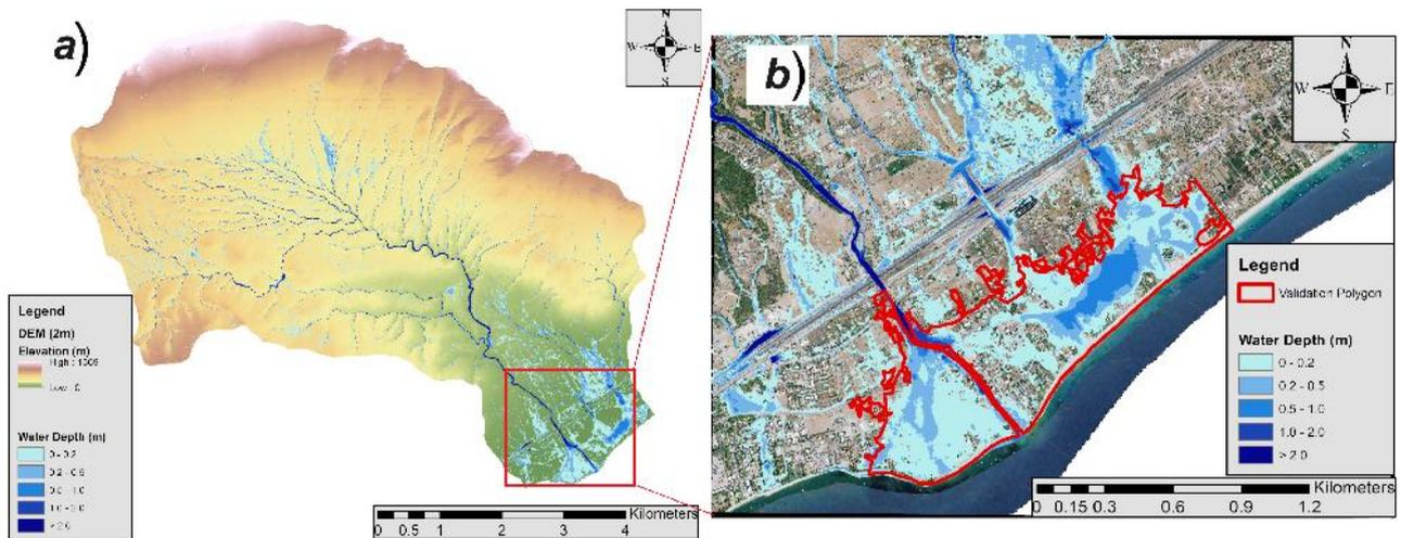
**Figure 5.** The hydraulic simulation results. (a) The extent of the flood in Kineta catchment; (b) The water extent and depth in the Kineta town. The red “validation polygon” represents the boundary of the water extent as resulted from RS analysis (shown in Figure 4d).
