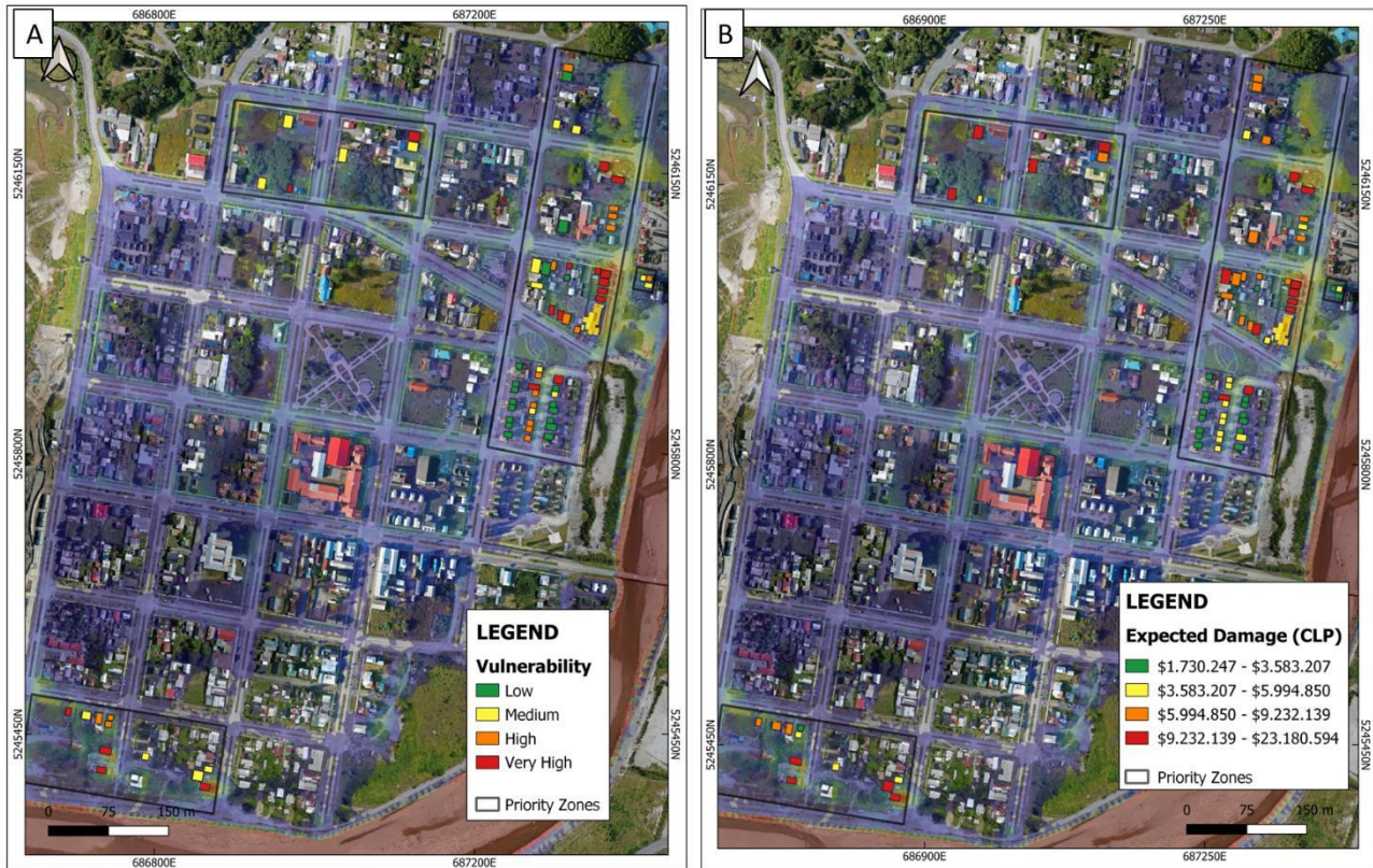
Figure 11. Vulnerability and Expected Damage maps. (A) Vulnerability Values per building; (B) Expected Damage values per building (damage in Chilean Pesos).
