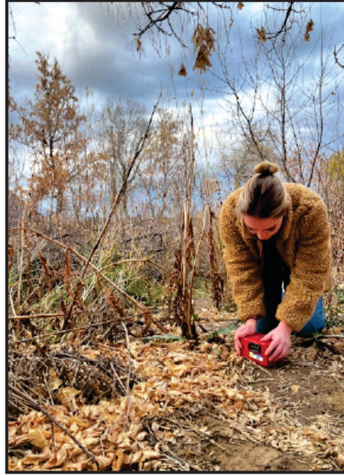
Figure 4. Photo showing the levelling of the seismometer and orienting it north at the “Spanish Oaks GC” field site ( Figure 2 and Table 1 ).
