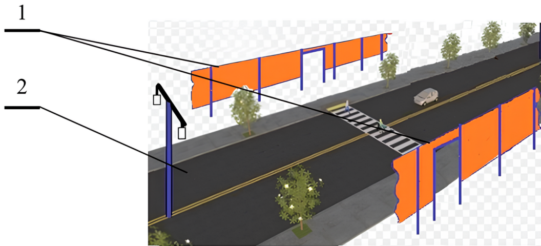
Figure 5. Lay-Out Diagram of Highway Development: 1 – The Fog Dispersion Machine; 2 – Roadbed.
