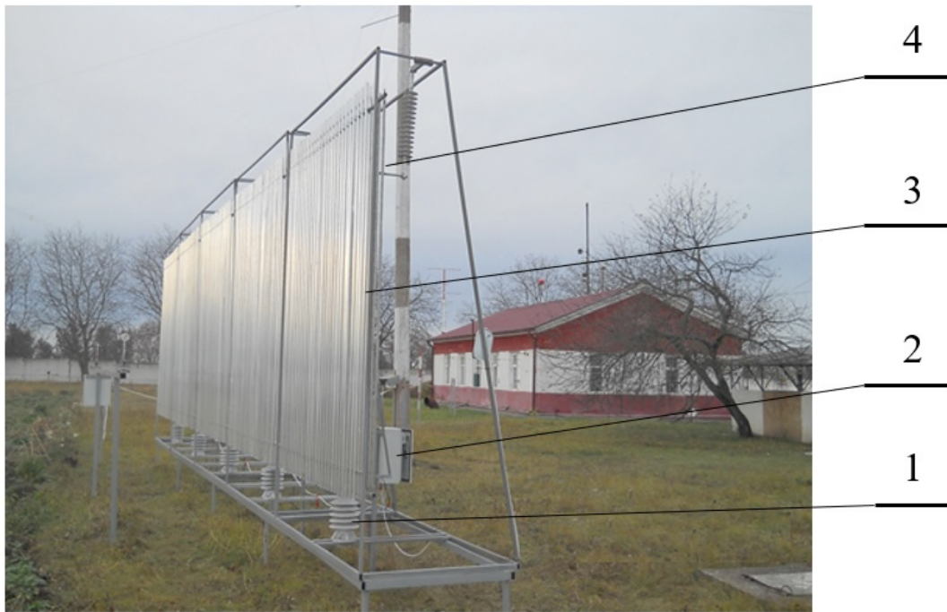
Figure 3. A Machine to Disperse Fog: 1 – High Voltage Insulator; 2 – High Voltage Power Supply; 3 – Grounded Electrodes; 4 – Corona Forming Electrodes.
