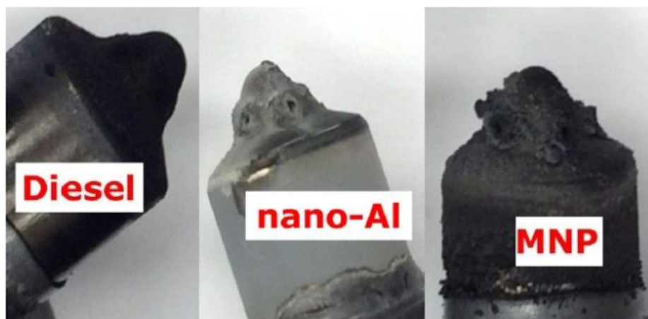
Figure 20. Images of injector tips for diesel and n-Al nanoparticles and Ti-Al-B metallic nanoparticles (MNP) mixture addition to JP5 fuel [34].
