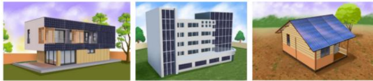
Figure 1. Building integrated photovoltaics (authors construct).
