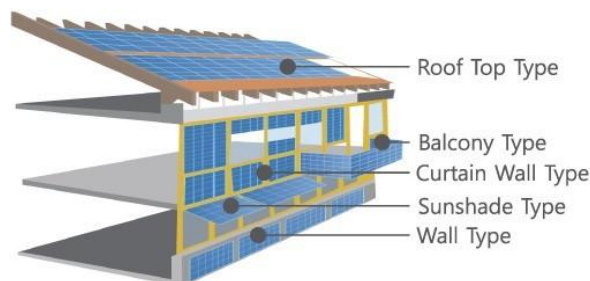
Figure 2. BIPV integration in buildings [26].
