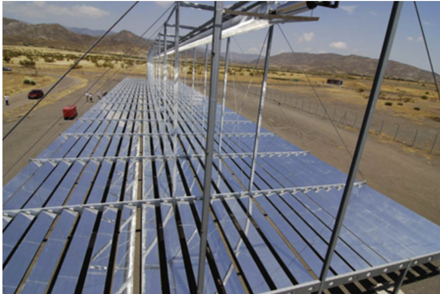
Figure 1. Linear Fresnel Test Collector Loop (FRESDEMO) at the Plataforma Solar de Almería, Spain [22].
