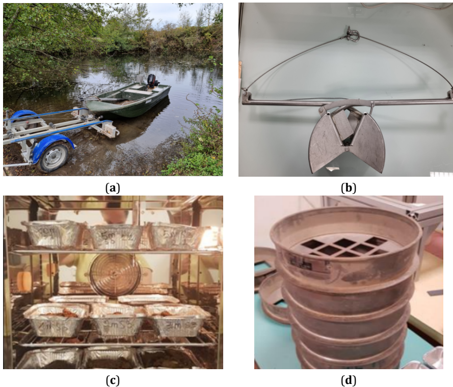
Figure 1. Equipment used to measure the sediment granulometry. (a) boat; (b) Van Veen sampler; (c) oven; (d) sieve column.
