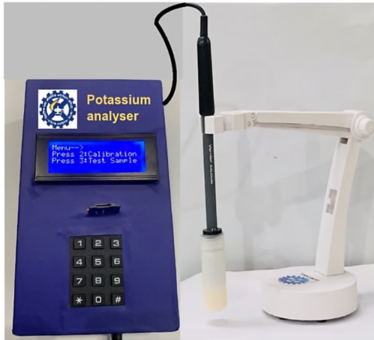
Figure 1. View of the developed soil nutrient analyzer.
