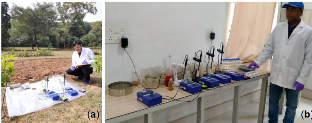
Figure 6. Soil nutrient analysis using ion-selective electrodes (ISE)-based soil nutrient analyzers (a) within agricultural fields and (b) in the laboratory at CIMFR, Dhanbad, India.
